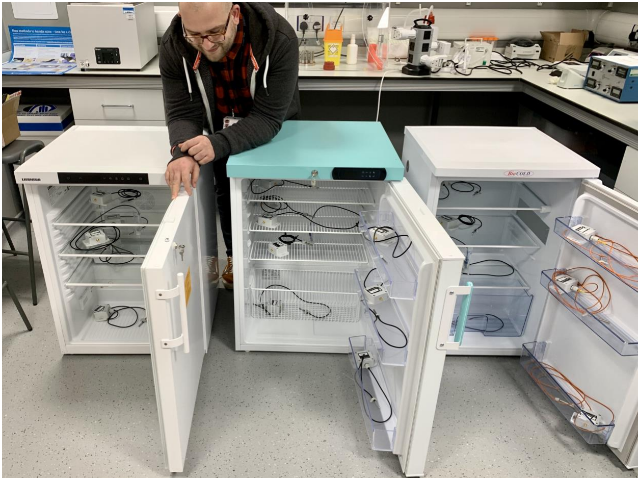
Figure 2. Each fridge with a temperature probe in each compartment together with a temperature probe placed in glycol at the centermost point to represent a sample. Dan Smith from the University of Birmingham holding open the Liebherr door which is self-closing.
