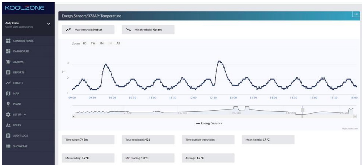
Figure 6. Lec door opening data from the sample probe. Door openings occurred at 9.39am and 12.28pm.
